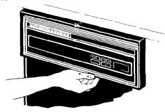
To stop the dishwasher, unlatch the door by pushing in the latch handle under the control panel. Do not open the door until the spray arms stop spinning. The DOOR OPEN indicator will flash and a tone will beep.
